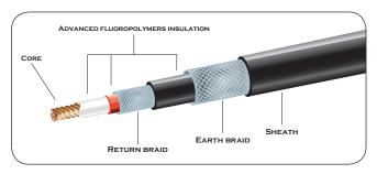
The product is designed for 240V supply installations- ensure the correct heater for the correct power supply has been purchased. Applications at 208V and 277V can be made effective with customized spacing of the heating cable. The cable produces between 10 to 20 Watts per sqft (100W to 200W/SQM) of heating, depending on the spacing of the cable (see Sizing Guide at the back of the manual). The product is CSA approved.
