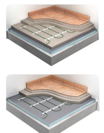
The subfloor of the project should be suitable for laying concrete. All normal requirements for laying concrete should be applied prior to installing the Warmup WODH systems.
