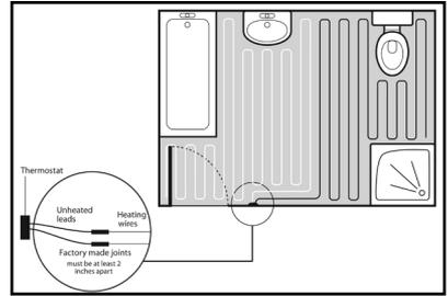
Marking the heating cable layout on floor plan makes it easier to trace back the heating cable for trouble shooting purpose. Keep such a layout filed after installation.
