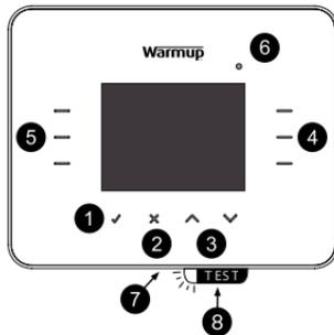
If you do not press any button on the thermostat for 1 minute, then it will go to standby mode. In standby mode the screen will be dimmed but the thermostat will continue to function as normal. To exit standby mode press "wake" (✓).
