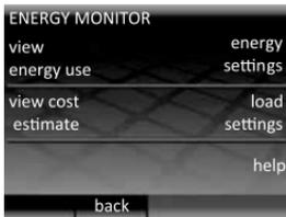
Your thermostat monitors the amount of energy your floor heating system is using, you can use these pages to view the amount of energy used and set parameters to estimate the cost of that energy.
