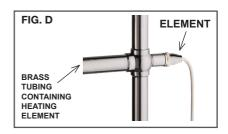
The Heating Element Hot and Neutral and green wire bond leads should be connected to the corresponding supply leads via a suitably sized UL listed wire nut.
