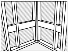
should be 1 inch above seat position for 2x4, 2 inches above for 2x6. This is to ensure that the attaching screws strike the optimal point in the blocking.
