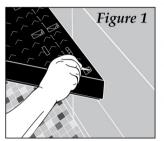
this exact placement.) Drill 3/8 inch holes through the tile and insert the supplied anchors by gently tapping flush to the tile surface. Use an adhesive caulk applied to the back
