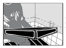
• A continuous bead of an adhesive caulk is to be applied on the back sides of the seat, where the seat contacts the wallboard.
