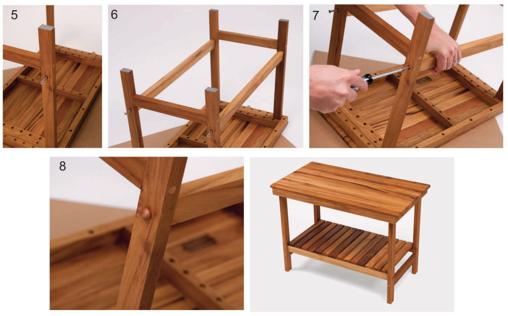
Use the provided Hardware Kit B (long screws), and screw the 2" screw through the leg so just a little bit sticks out (about  $\frac{1}{6}$ ")(5). Repeat on all sides of the 4 legs (6). Place the spanners onto the screws and then tighten both screws on legs, then do opposing side legs (7). **The long side of spanner should run vertical**
